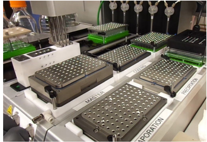
Heated filter block on temperature controlled station
