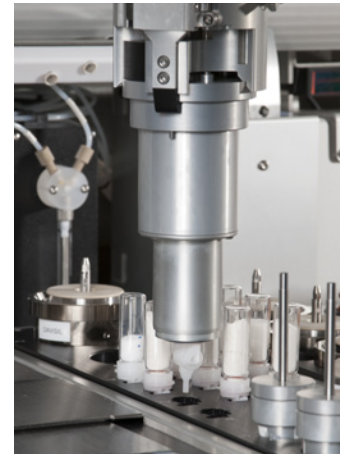
SV dispensers use vibration for precise delivery
