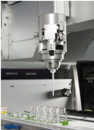
Viscous liquid dispenser handles up to 1000 cP
